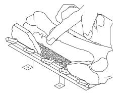
Figure 57 - Placing Ember Material on Burner
